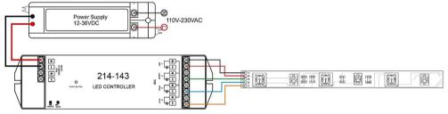
2)Receiver Connection Diagram for Multiple Units
